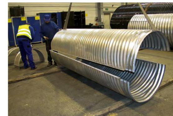
Flexible, cold formed helically corrugated steel pipes, produced as bifid pipes (half pipes), bolted together with L-shape steel elements and longitudinally connected with couplings, can be used in as a steel-soil structures under road and railways loads.
