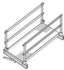
Cantilevered walkways with the width of 1.5 m, located outside the truss panels ensure separation of pedestrian traffic from the vehicular traffic, which increases the safety of pedestrians.
