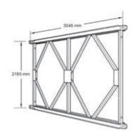
Truss panels with the dimensions of 218.50 cm x 304.80 cm joined together with the use of bolts
