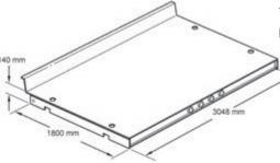
Steel decks placed on the crossbars ensure the possibility of vehicular traffic. Surface of the bridge deck in the form of steel plate or steel plate with epoxy coating applied in the factory. It is also possible to make a wooden deck. Fixing the decks to crossbars is very simple and takes place from the level of the deck with the use of bolts
